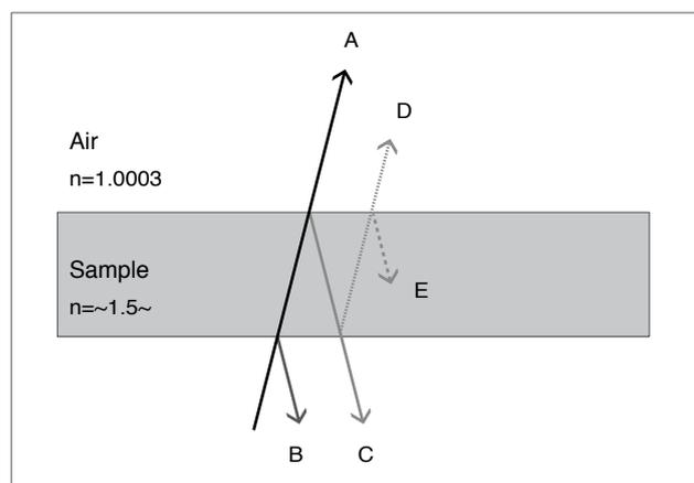
Fig. 2 Overview of Transmission Method
