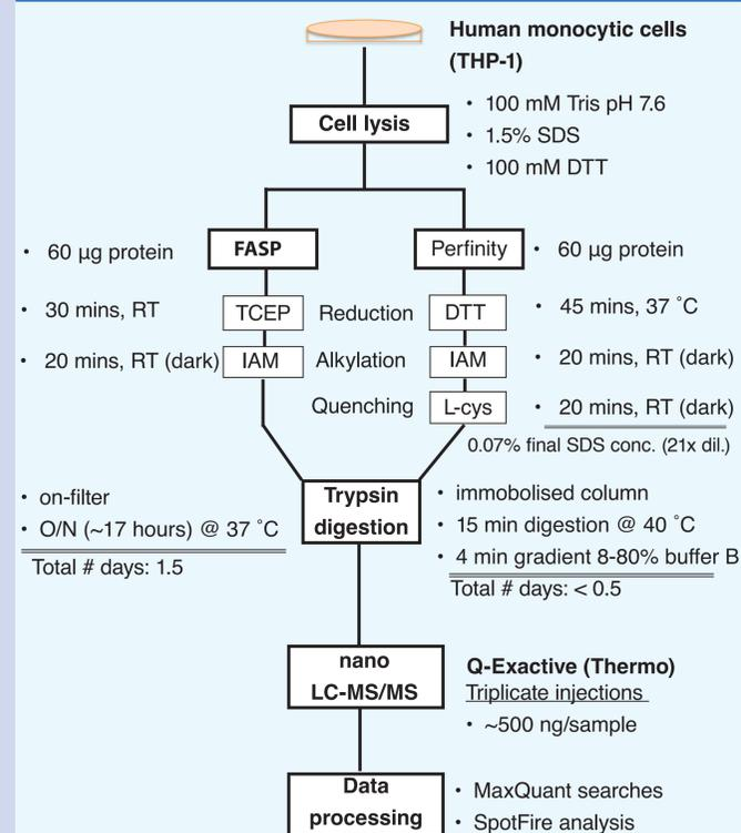
**Figure 2:** Workflow illustrating the methodology used in this study to compare the FASP protocol with the online trypsin digestion procedure via the Perfinity LC system. In this study human monocytic cells (THP-1) were first solubilised in a buffer containing 1.5% SDS and digested at 0.07% final concentration<sup>2</sup> prior to performing on-column trypsin digestion.
