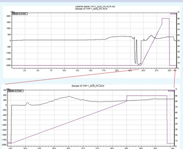
**Figure 3:** Chromatographic UV absorbance traces of the THP-1 cell lysate subjected to trypsin digestion on the immobilised column using the Perfinity LC workstation. Inset: a zoomed in version of the trace illustrating the increase in UV absorbance detected between 25-28 mins representing the peptides that were eluted off the RPC column (in line with the trypsin column) and collected for subsequent MS analysis.
