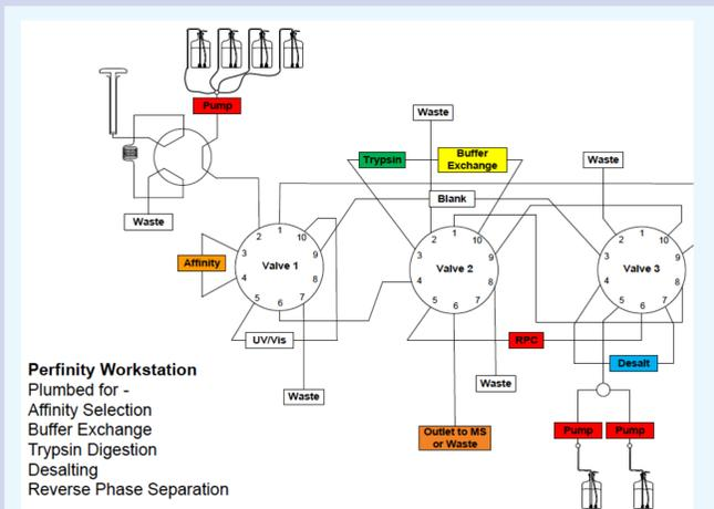
**Figure 1:** Schematics of the LC configuration for the Perfinity workstation based on the Shimadzu™ modular HPLC system.
